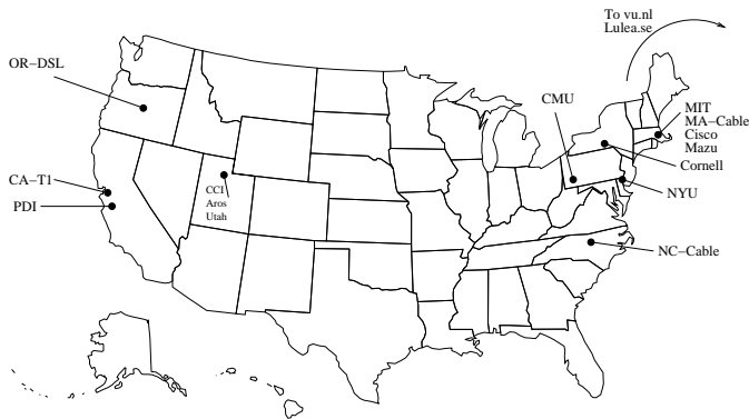
Figure 1: The current sixteen-node RON deployment. Five sites are at universities in the USA, two are European universities (not shown), three are “broadband” home Internet hosts connected by Cable or DSL, one is located at a US ISP, and five are at corporations in the USA.
